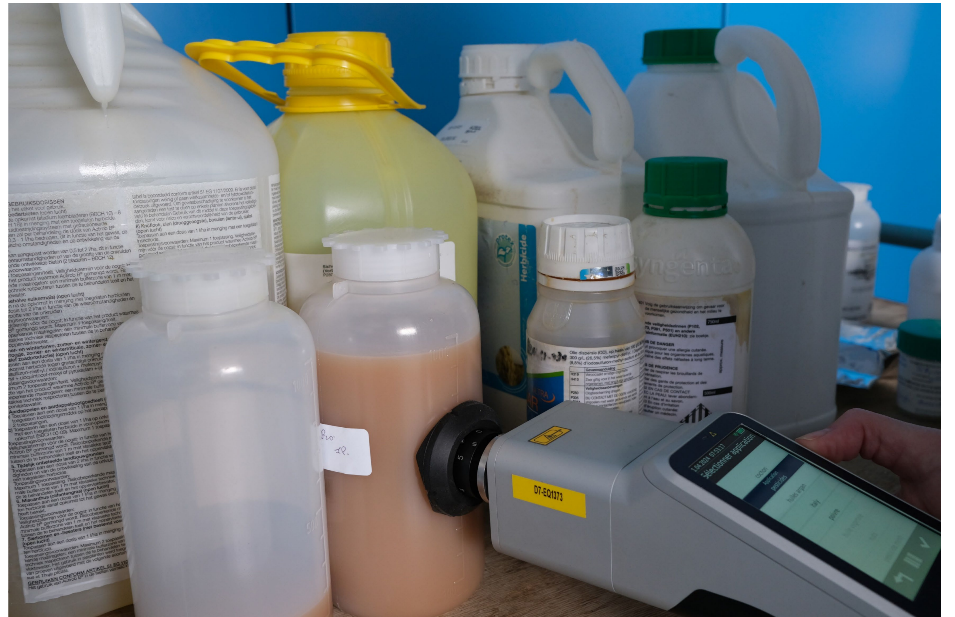
An hypothetical situation ? Measurement of a pesticide formulation using a portable Raman device in a warehouse
